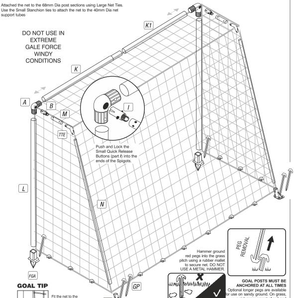
for use on sandy ground. On grass, a risk assessment of soil and eather conditions suitability should be carried out when anchors are to be used. Extra anchors are available TFI : 0114 2424244
