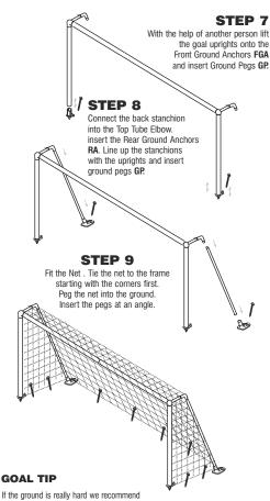
adding water to the ground to soften Also use a wooden block or dowling to help insert your anchors into the turf. ALWAYS Use a rubber mallet not a metal hammer.
