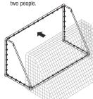
STEP 3 Attach the corners first, where the upright posts meets the crossbar as shown. Then attach the net to the post using the net fixings
