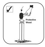
ALWAYS USE A PROTECTIVE PIECE OF WOOD (NOT INCLUDED) BEFORE HAMMERING THE TOP OF THE METAL SPIKE.
