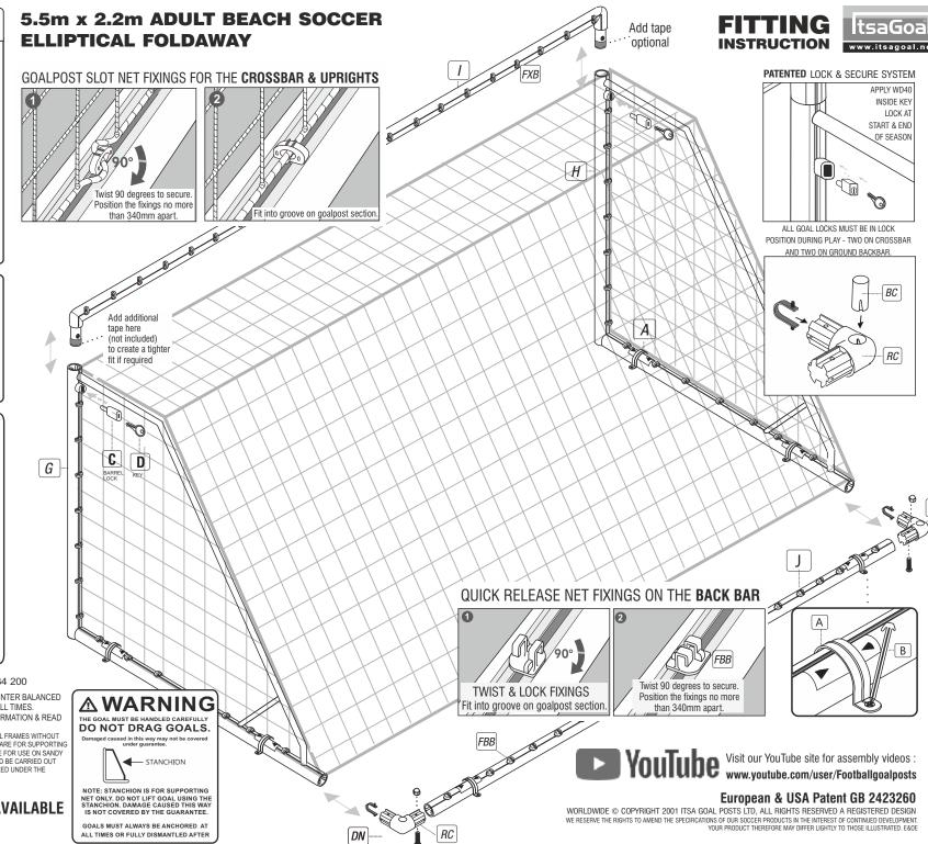
Lockable aluminium folding patented goal posts that are easy to move around use and store. Crossbar corners are welded both internally and externally to ensure they will stand up to the most rigorous conditions. The corners will not expand apart as with other goals as expansion is carried through the corner to lift the crossbar slightly and then when contracting gravity will take over.
