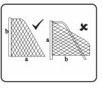
SQUARE MESH Net is cut to shape Simply throw over the frame and fit each end onto top stanchion by securing on each corner of crossbar.
