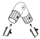
Push and Lock the Large Quick Release Buttons into the ends of the Corner Brackets.
