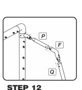
Join top tubes P to elbows F and back tubes Q and connect to the goalpost
