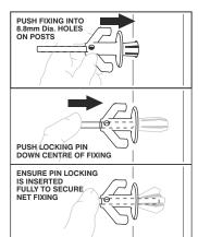
INSERT NET FIXINGS INTO HOLES ON REAR OF GOAL. A LOCKING PIN IS LOCATED ON THE TOP OF THE NET FIXING.
