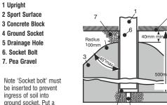
`5 dab of grease on it and insert the screw into the hole and just leave it in place. At any time in the future it can be locked'
