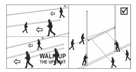
With a minimum of 6-8 people, two people will need to hold down the bottom of the goal section to stop it from sliding. Another two people will need to walk up the uprights on each side to erect and place into position over the ground. It is also recommended to use guide ropes as shown for additional safety.
