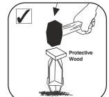
ALWAYS USE A PROTECTIVE PIECE OF WOOD (NOT INCLUDED) BEFORE HAMMERING THE TOP OF THE METAL SPIKE.
