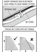
SQUARE MESH Net is cut to shape Simply throw over the frame and fit each end onto top stanchion by securing on each corner of crossbar. NOTE: If your net does not fit the first time. you may be fitting it to the goal frame upside down i.e. that is to say the net from the crossbar to the floor (a) is longer than the length of the net to the bottom of the upright (b).
