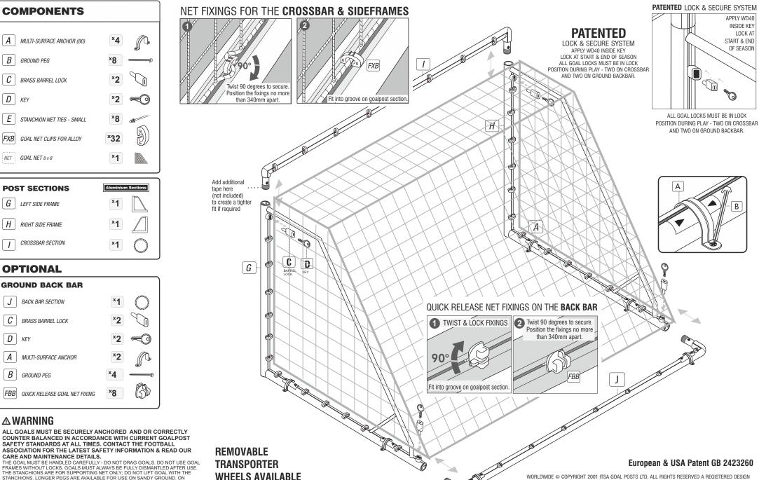
THE STANCHIONS ARE FOR SUPPORTING NET ONLY: DO NOT LIFT GOAL WITH THE STANCHIONS, LONGER PEGS ARE AVAILABLE FOR USE ON SANDY GROUND, ON GRASS, A RISK ASSESSMENT OF SOIL CONDITIONS SUITABILITY SHOULD BE CARRIED OUT WHEN ANCHORS ARE TO BE USED. ANY DAMAGE CAUSED BY MIS-USE IS NOT
