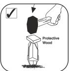
ALWAYS USE A PROTECTIVE PIECE OF WOOD (NOT INCLUDED) BEFORE HAMMERING THE TOP OF THE METAL SPIKE.
