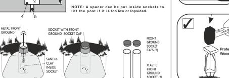
**OPTIONAL EXTRA GROUND SOCKET** When an upright post is anchored in the same position
