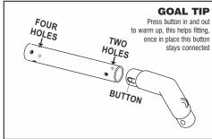
NOTE: Ensure that the two holes of the stanchion are parallel to the buttons of the Top Tube Elbow before connecting.
