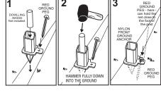
With the crossbar laid on the floor insert the Front Ground Anchors FGA as shown, this will provide the correct distance between the posts for the anchors to be inserted. Ssee the Goal tip. right.
