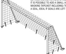
Connect the back stanchion into the Top Tube Elbow. insert the Rear Ground Anchors RA. Line up the stanchions with the uprights and insert ground pegs GP.
