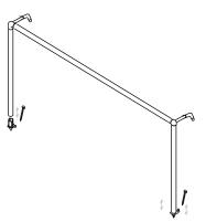
With the help of another person lift the goal uprights onto the Front Ground Anchors FGA and insert Ground Pegs GP.
