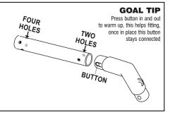
NOTE : Ensure that the two holes of the stanchion are parallel to the buttons of the Top Tube Elbow before connecting.
