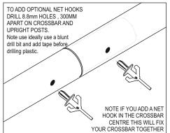
NET TIES : Place the small stanchion net ties on the net support stanchions. This will help extend the life of your net and keep the frame tightly fitted together. Apply the larger ties to the ground frame and the posts. We recommend placing the net ties no more than 340mm apart. The net ties supplied are designed to permanently fix the net to the goal frame. If you require to take nets on and off, other net fixings can be used.
