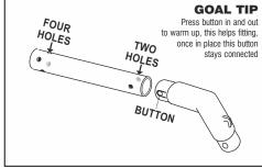
NOTE: Ensure that the two holes of the stanchion are parallel to the buttons of the Top Tube Elbow before connecting.
