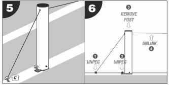
1. On the last barrier post use a tension peg to complete your barrier system and reinforce stability. To dismantle simply start at one end and follow the steps in reverse order un-peging and un-linking the posts (steps 5 - 6).
