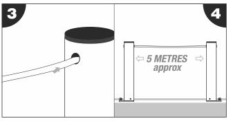
1. Attach your own rope into pre drilled holes. You will need approximately 5 metres of rope between posts.
