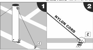
1. With your first barrier post in position use the tension peg to reinforce stability before assembling the rest of the barrier pack. Always start erecting the barrier from one side for an easy and efficient assembly (steps 1 - 2).
