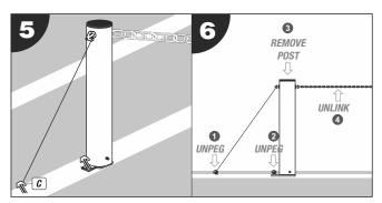
1. On the last barrier post use a tension peg to complete your barrier system and reinforce stability. To dismantle simply start at one end and follow the steps in reverse order un-peging and un-linking the posts (steps 5 - 6).
