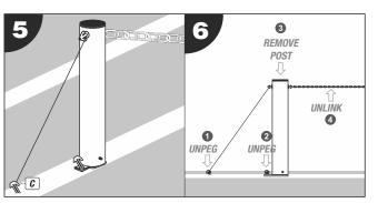
1. On the last barrier post use a tension peg to complete your barrier system and reinforce stability. To dismantle simply start at one end and follow the steps in reverse order un-peging and un-linking the posts (steps 5 - 6).
