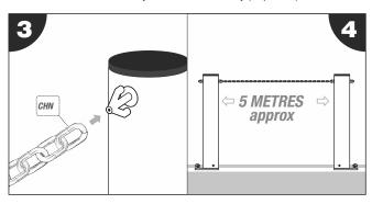
1. Attach your first chain link onto the arrowhead fitting. You will need approximately 5 metres of chain link per post distance (steps 3 - 4).
