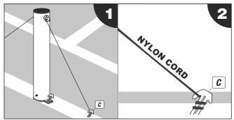
1. With your first barrier post in position use the tension peg to reinforce stability before assembling the rest of the barrier pack. Always start erecting the barrier from one side for an easy and efficient assembly (steps 1 - 2).
