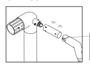
NOTE: Ensure Top Stanchion holes are aligned with the Stanchion Elbow.
