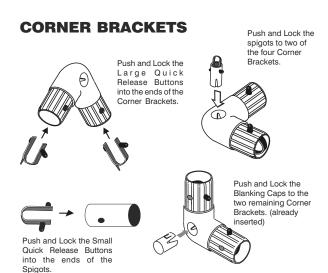
NOTE: All plastic extrusions vary and therefore some tubes may be looser or tighter to connector fittings. If you want to increase the diameter of the fitting just wrap masking tape around the part that fits into the tube, twist as you insert the fitting and it will grab to the tube tight ... you can make tighter fits by adding more tape.
