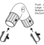
Push and Lock the Large Quick Release Buttons into the ends of the Corner Brackets.
