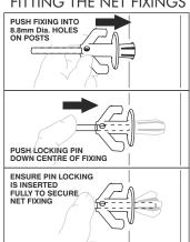
INSERT NET FIXINGS INTO HOLES ON REAR OF
