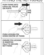
INSERT NET FIXINGS INTO HOLES ON REAR
