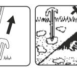
INSERT SEPARATE ROD IN BETWEEN EACH FIXING TO LOCK TO POST
