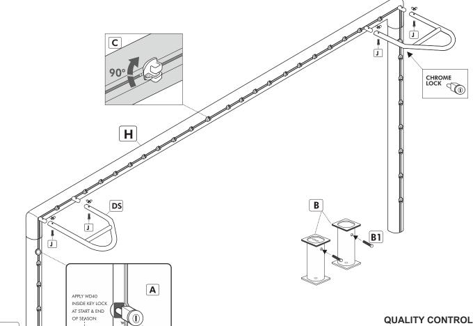
For quality control each goalpost is assembled before despatch. This is to ensure alignment of fixing positions and so customers can be assured their goalpost will assemble. The corners and fixing joints are marked and should be matched up as they are individually made by craftsmen and assembled in the workshop before despatch. If you have multiple goals of the same type the numbering is the final quality control check before goal posts are despatched.
