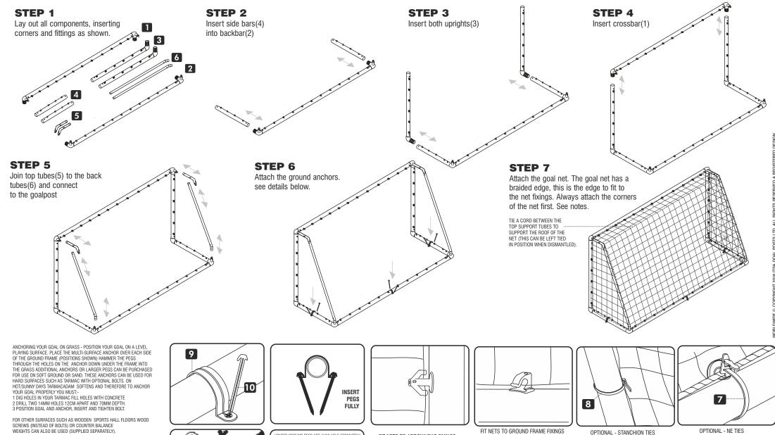
WARNING: Check the position of any underground services before using the ground anchors and pegs. We take no responsibility for any damage or injury caused in this manner. Our ground anchor system is designed to give slightly under heavy impact to help prevent serious injury. To loosen tap sides of the nylon ground anchor with a hammer before extracting.
