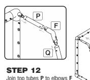
Join top tubes P to elbows F and back tubes Q and connect to the goalpost.
