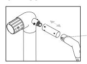
NOTE: Ensure Top Stanchion holes are aligned with the Stanchion Elbow.
