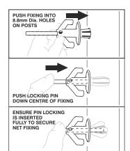
INSERT NET FIXINGS INTO HOLES ON REAR OF GOAL. A LOCKING PIN IS LOCATED ON THE TOP OF THE NET FIXING.
