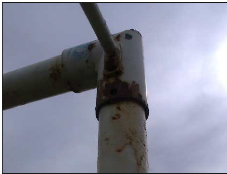
Figure 45 Old fashioned nut & bolt goals soon end up like this - not itsa goal anti vandal goal posts (not an ITSA goal product).
