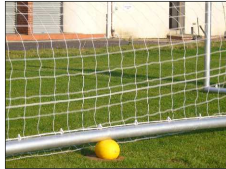
Figure 1 The 70mm dia. lightweight goal post was dropped on the melon three times and showed only very slight bruising.
