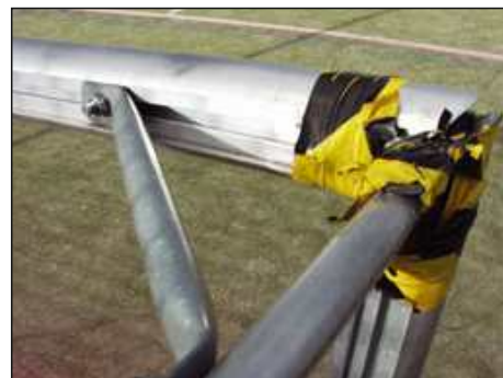
Figure 30 Others mitred corner Goal post on free standing oval goal with rear rollers (not an ITSA goal product).
