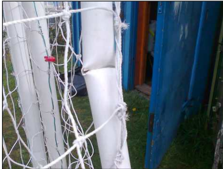
Figure 20 Samba goal net support tube showing why many end up with out net supports.
