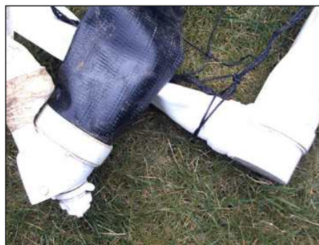
Figure 3 Superglue & industrial tape repairs on joints after four matches.
