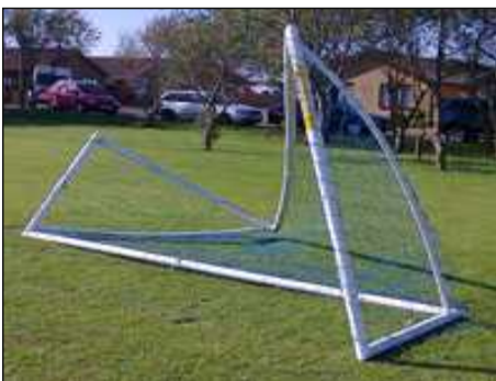
Figure 22 The twisting nature of far-east goalposts.
