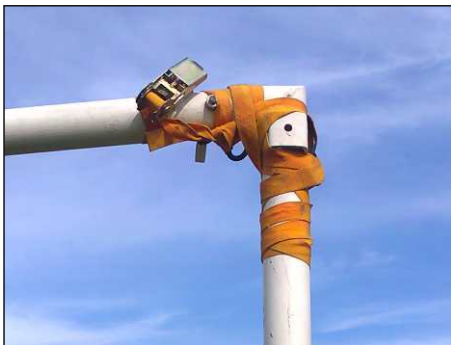
Figure 45 Old fashioned nut & bolt goals soon end up like this - not itsa goal anti vandal goal posts (not an ITSA goal product).
