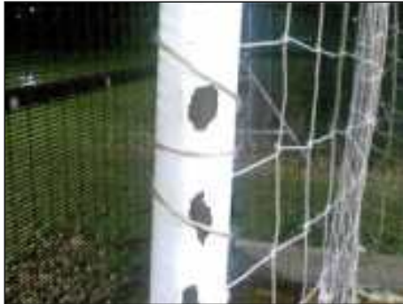
Figure 40 Photograph shows the problems and damage to paintwork that have nets pulled and clipped around the front of the goal post uprights (not an ITSA goal product).
