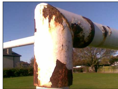
Figure 38 The type of protruding corner found on basic steel nut & bolt football goal posts (not an ITSA goal product).
