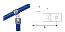
A versatile swivel fitting, useful for awkward applications where angles cannot be accommodated by adjustable angle fittings. The through tube (sloping in photo) cannot be joined within the fitting. The assembly is riveted together, although items can be supplied separately as 173M and 173F.
