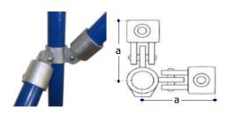
A versatile swivel fitting, useful for awkward applications where angles cannot be accommodated by adjustable angle fittings. The through tube (vertical in photo) cannot be joined within the fitting. The assembly is riveted together, although items can be supplied separately as 168M and 2 x 173F.
