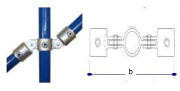
A versatile swivel fitting, useful for awkward applications where angles cannot be accommodated by adjustable angle fittings. The assembly is riveted together, although items can be supplied separately as 167M and 2  $\times$  173F. The through tube (vertical in photo) cannot be joined within the fitting.
