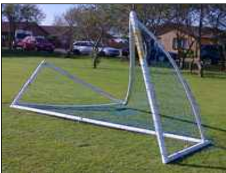
Figure 22 The twisting nature of far-east goalposts.
