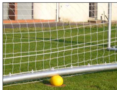
Figure 1 The 70mm dia. lightweight goal post was dropped on the melon three times and showed only very slight bruising.
