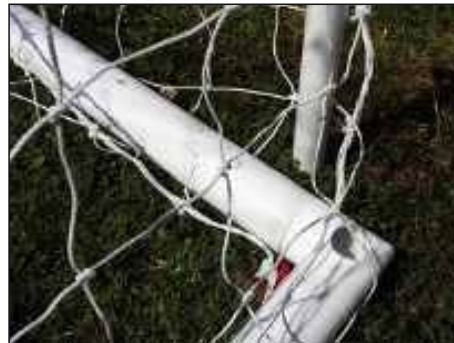
Figure 26 Samba Match goal post with net support stanchion just pushed into a hole and not secured.
