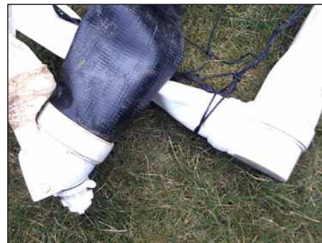
Figure 3 Superglue & industrial tape repairs on joints after four matches.
