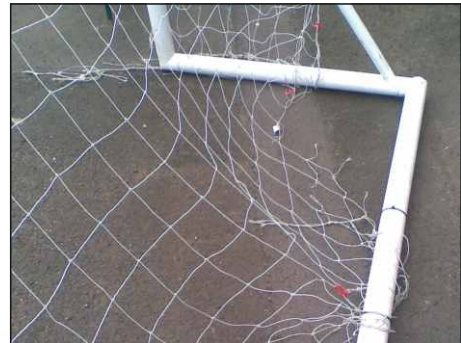
Figure 23 Samba Goal showing how quickly the net frays due to being wrapped around base of posts.
