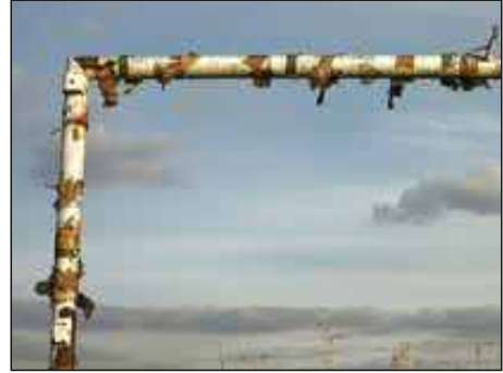
Figure 47 A Nut and Bolt steel socketed goals without net fixings eventually end up with the net being pulled of the posts (not an ITSA goal product).
