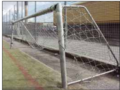
Figure 36 Badly designed mitered corner Aluminum goal (not an ITSA goal product).
