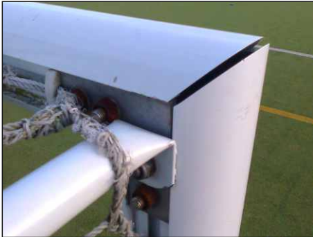
Figure 32 Adult Five-A-Side goal with rollers - continually being loosened when moved (not an ITSA goal product).
